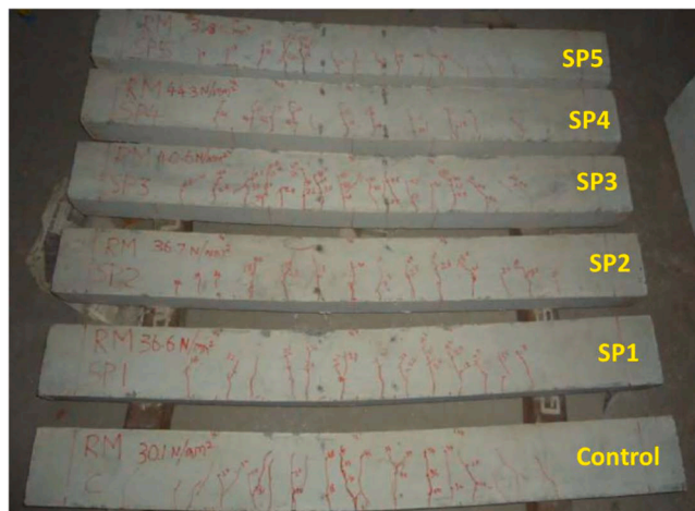
Fig. 22. View of crack and failure patterns of the tested concrete specimens.
