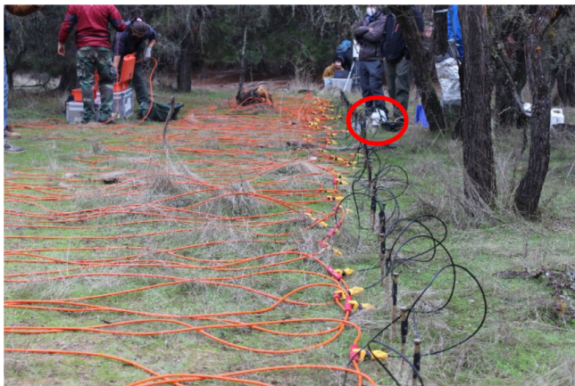
FIGURE 1 The study site. At the center (red circle) is found the EnviroSCAN, Vachellia caven tree, and the infiltration ring in between two electrodes. At the bottom of the picture is the Pinus plantation.
