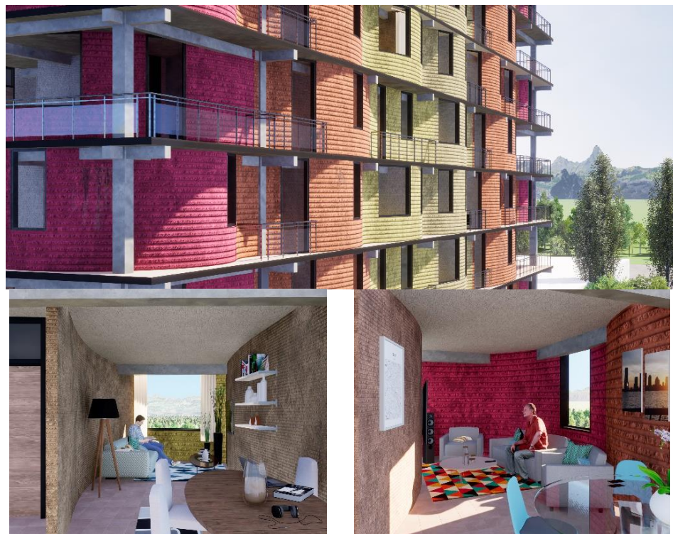
Figure 6. Rendered view of outdoor and indoor spaces with main structure of reinforced concrete slabs and columns, and 3D-printed walls (Source: authors).
