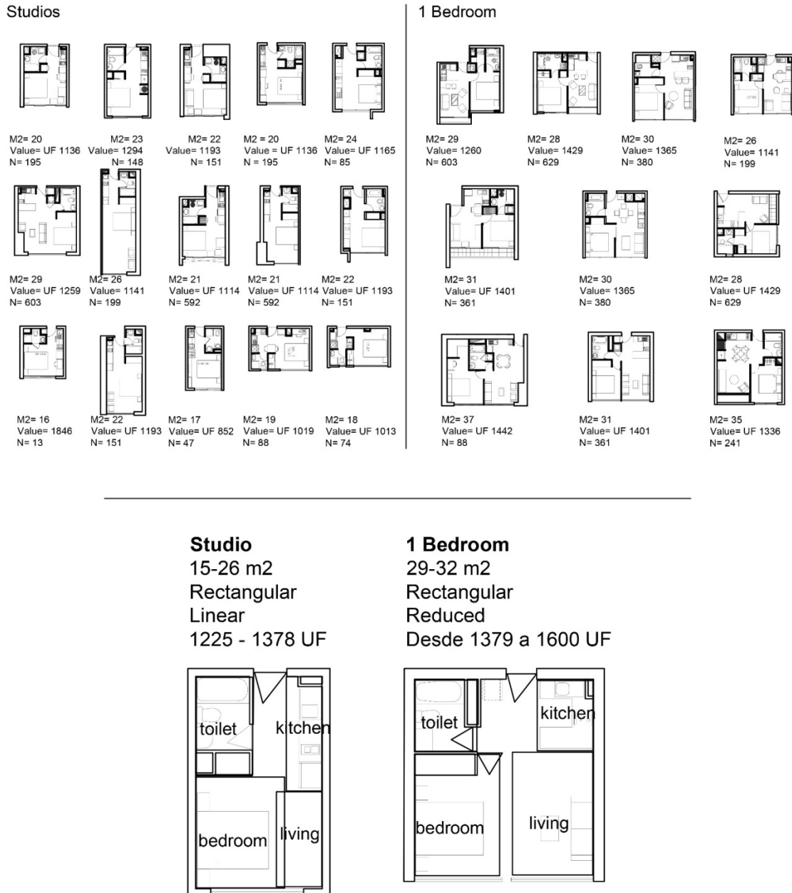
Figure 3. Synthesis of planimetries analyzed and typological results of the housing unit financed in the verticalization model.
