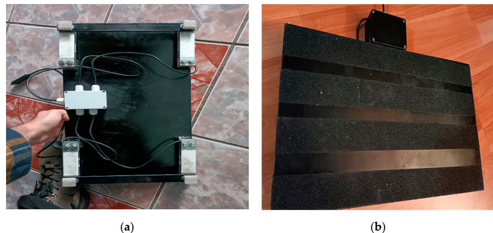
Figure 1. Bottom view (a) and top view (b) of the G-Force force platform with YZC-516 load cell.
